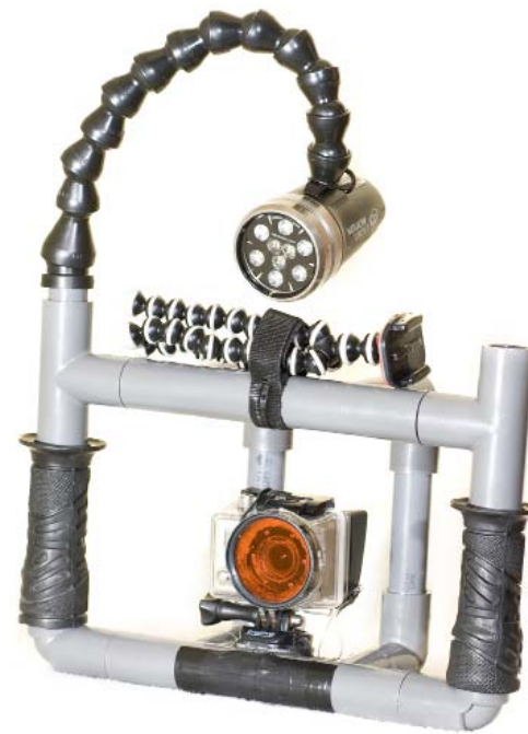
A bit of PVC pipe and some bike grips and you have a sturdy base to hold on to, mount accessories on, and protect the camera with.
