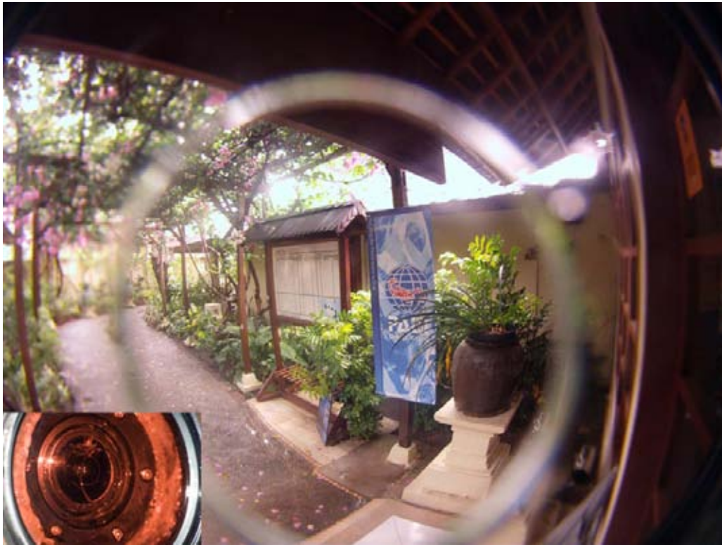
Photo taken using my refocused gopro, with a drop of water between the dome and a red filter. Note that the area of the image that was shot through the water is in focus.
