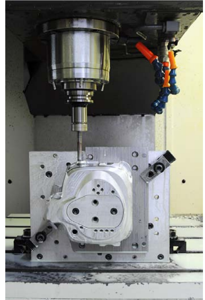
High precision machinery machines housings from a solid block of aluminium.
