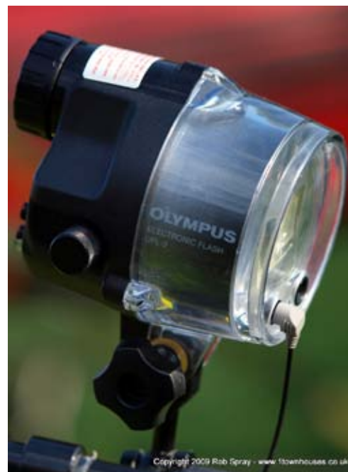
The UFL-2 is an incredibly light and compact TTL underwater flash that is waterproof to 60 metres.
