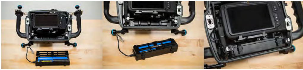
Four 18650 batteries greatly extend the runtime of the BMPCC4K
